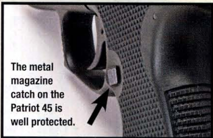
The triggerguard of the Patriot 45 is ample, with grooving on it and the trigger. The finger grooves aid in controlling recoil.
