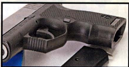
The triggerguard of the Patriot 45 is ample, with grooving on it and the trigger. The finger grooves aid in controlling recoil.
